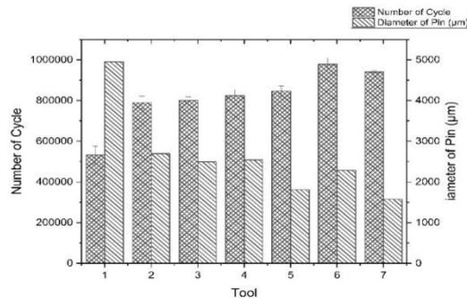
Figure 5. Chart depicting the relationship between Pin Diameter and Number of Cycles
