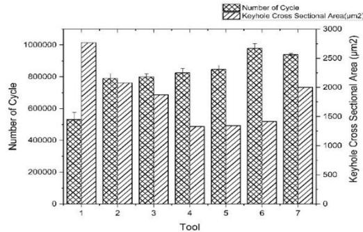
Figure 4. Keyhole cross-sectional area chart plotted against the number of cycles
