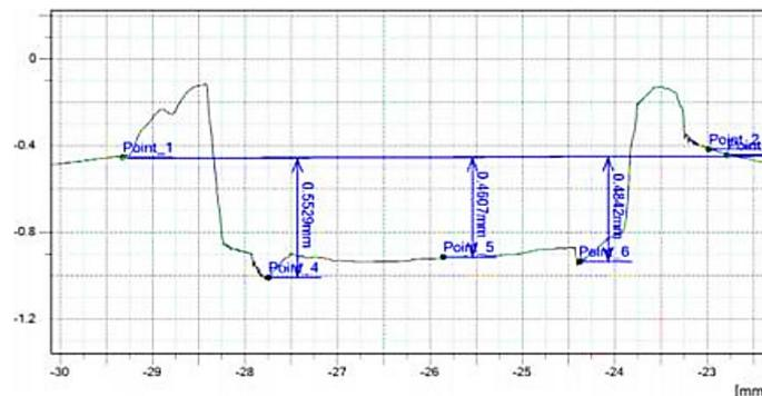
Figure 3. Contour of Weld Result Obtained with Tool 1
