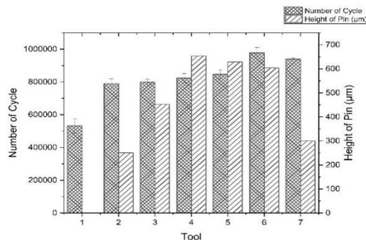
Figure 6. Chart depicting the relationship between Pin Height and Number of Cycles
