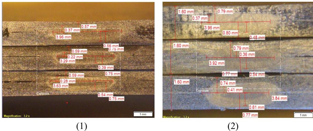
Figure 8. Diameter values of spot-welding specimens (1) 0.8 + 0.6 mm thickness, (2) 0.8 + 0.8 mm thickness
