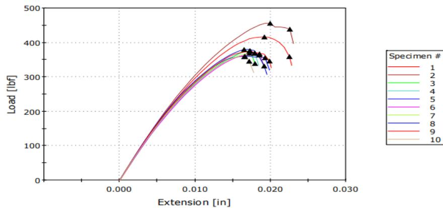
Figure 7. Graph of tensile test with 0.8 + 0.8 thickness
