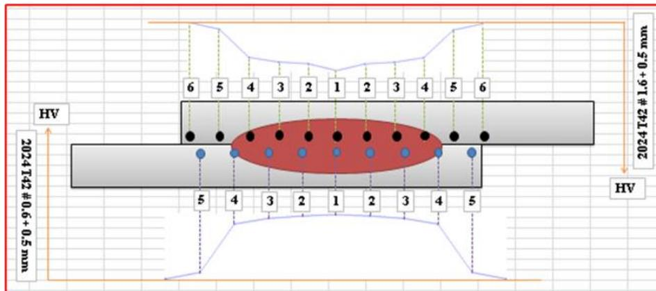
Figure 11. Hardness value distribution graph
