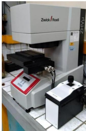
Figure 5. Machine Hardness test
